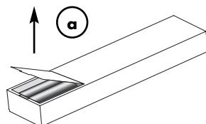
b) If necessary, remove used batteries and insert new ones correctly as shown by the diagram in the battery compartment.
