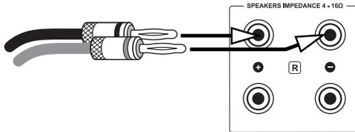
If you want to use speaker cables equipped with spade lug connectors, every connector screw must be opened by turning counter clockwise. After that, the lug must be moved under the screw head. Then, turn the screw clockwise to fasten the lug to the connector. To avoid damages to the amplifier, make sure the connection is tight and no bare metal from the cable lug connector makes contact with the rear panel or with another terminal.
