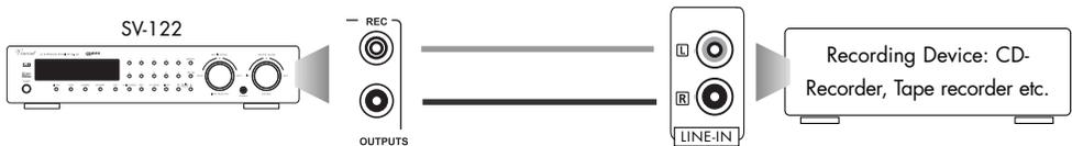
Connect this signal output of the preamplifier using RCA cables to the signal input („RECORD“ or „INPUT“) of the recording device. It is possible to connect other devices that accept the line level signal of the source that is selected at the receiver (for example integrated amplifiers).
