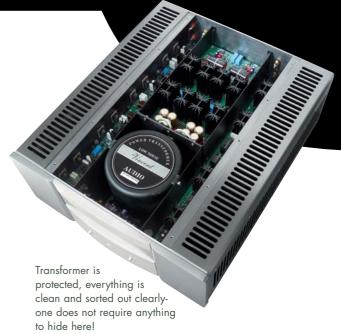
In each case, the signal is taken from the FET differential- input amplifier and reaches in the most direct way to the 16 power transistors of the output. This task of amplifying the signal is then supported by 6000uF electrolytic capacitor per channel.
